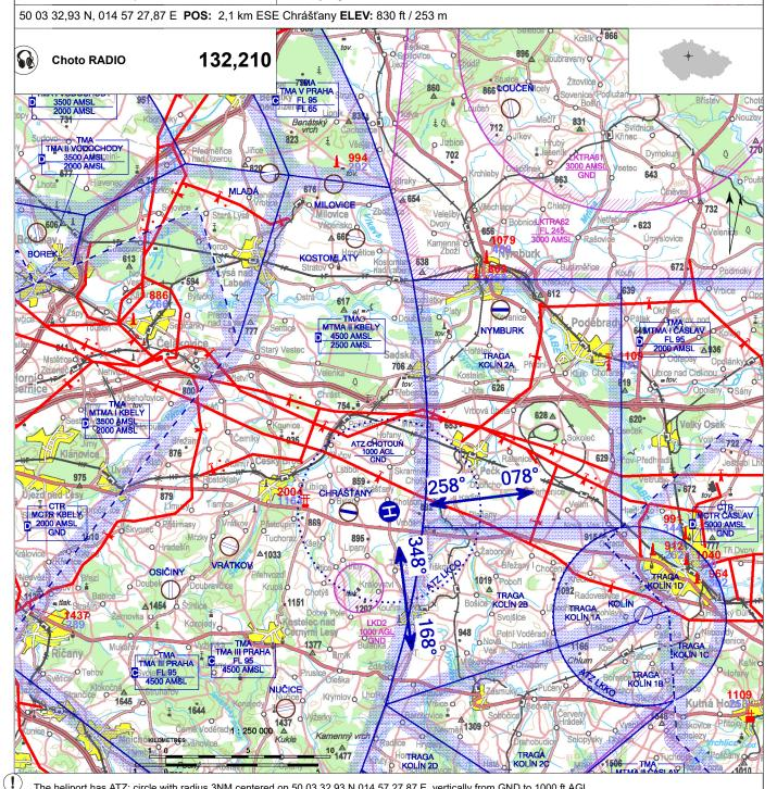
The heliport has ATZ: circle with radius 3NM centered on 50 03 32,93 N 014 57 27,87 E, vertically from GND to 1000 ft AGL. ATZ penetrated by LKD2 area.
